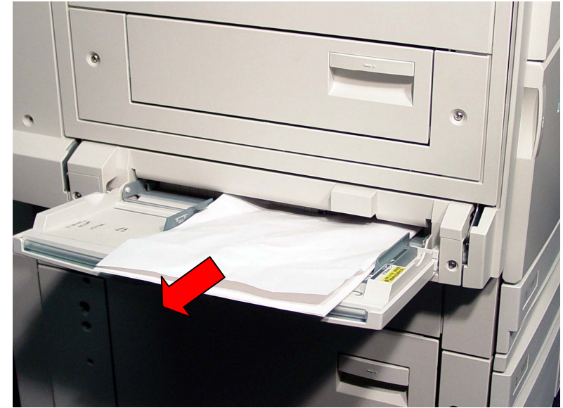
Fig. 6 Tray 5 (Bypass) Inspect the inside (paper feed entrance) of Tray 5 (Bypass), and remove any jammed paper.
