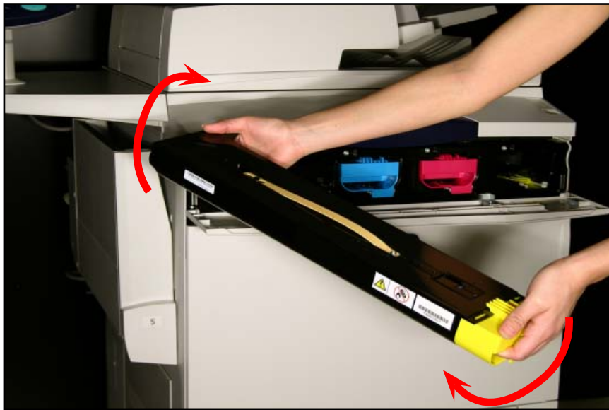
Fig. 4 Lightly shake the "new" toner cartridge three or four times up and down and to the left and right.
