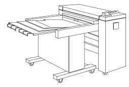
The Stacker 1000 stacks a maximum of 1000 prints of various sizes. Print sizes include A (A4) through E (A0). Depending on the print size, prints are stacked either by:
