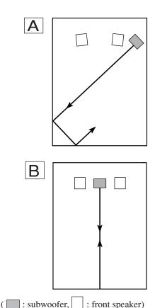
It is recommended to place the subwoofer on the outside of either the right or the left front speaker. (See fig. A.) The placement shown in fig. B is also possible, however, if the subwoofer system is placed directly facing the wall, the bass effect may die because the sound from it and the sound reflected by the wall may cancel out each other. To prevent this from happening, face the subwoofer system at an angle as shown in fig. A.
