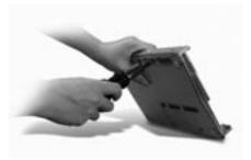
**5.** Replace top cover and make sure it is aligned with bottom cover.
