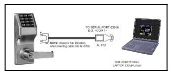
**Application 1** Program the Lock directly using a PC or Laptop
