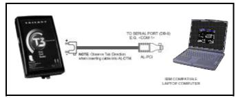
**Application 3** Connect the AL-PRE Prox Card Enroller to the PC to read Prox Cards directly into DL-Windows.
