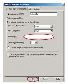
**Important:** A WEP key is a mixture of numbers and letters from A–F and 0–9. For 128-bit WEP, you need to enter 26 keys. For 64-bit WEP, you need to enter 10 keys. This network key needs to match the key you assign to your wireless router or access point.
