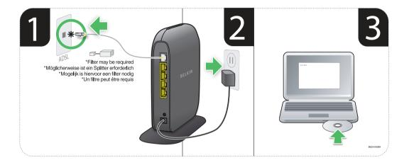
Connect your Router's ADSL cable to your phone jack or phonejack adapter (microfilter). If you are replacing an existing Router or gateway, this may require unplugging the existing gateway.
