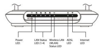
1.6 Turn on your computers. After your computers boot up, a LAN status LED on the front of the Router will light for each port to which a wired computer is connected. These LEDs indicate connection and activity status. Now you are ready to configure the Router for ADSL connection.
