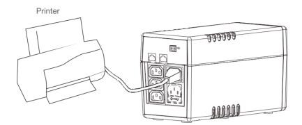
Note: DO NOT plug a laser printer, copier, space heater, vacuum or other large electrical device into the UPS. The power demands of these devices will overload and possibly damage the unit.
