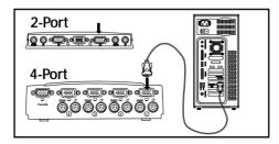
5. Connect the first computer's PS/2 keyboard and PS/2 mouse cable to the appropriate ports on the section labeled CPU1. (Belkin Part# F3X1105-XX, F3X1835-XX, or F2N036-XX).
