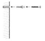
Step 5. Place screws into anchor until 10mm is still visible.
