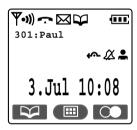
Ψ Within range of a Cell Station **ΫΨ**( Out of range, No registration •))) Intercom Indicator **Off-hook Status** Message Waiting  $\square$ Phonebook Mode  $\square$ Battery Strength Hot Line ON X **Ringer Volume OFF** N Vibration Μ Meeting Mode Call Forwarding ŝ Do Not Disturb •<del>K</del>—
