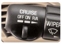
The Cruise Control feature is located at the end of the Turn Signal/Multifunction Lever. Cruise Control allows you to maintain a speed of about 25 mph or more (but not below 25 mph) without keeping your foot on the accelerator. To use Cruise Control:
