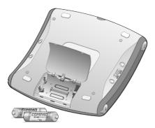
**Tip:** To recharge the batteries that came with your PCD-1, just plug the PCD-1 into a standard electrical outlet while the batteries are in the battery compartment. The battery icon on the display screen shows the amount of charge held by the batteries (when the PCD-1 is not plugged into an AC electrical outlet).
