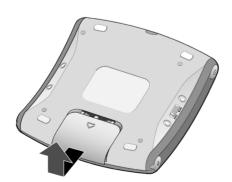
2. Place the rechargeable batteries that came with your PCD-1 into the battery compartment according to the diagram inside the compartment.
