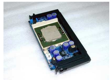
The processor after applying thermal compound.
