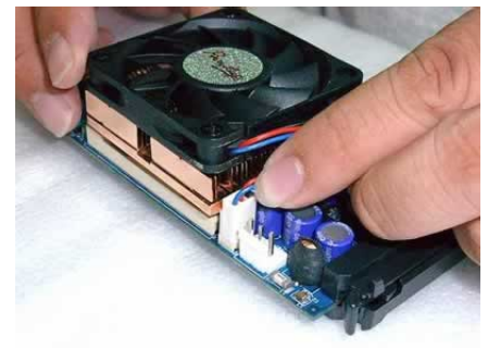
Connecting the fan's power cable to the PL-P3/SMP.
