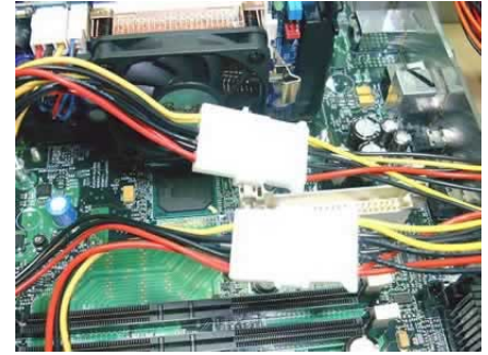
The connected cables for two PL-P3/SMPs.
