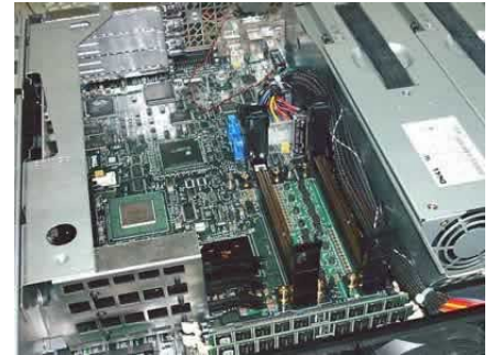
After removing both original processors. We recommend using a small brush to remove any dust from the slots.
