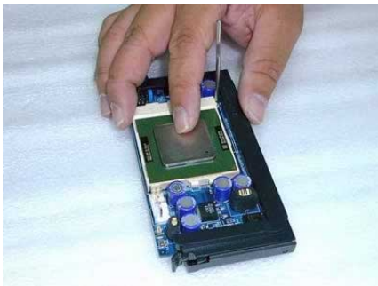
Installing the processor in the PL-P3/SMP. (1)
