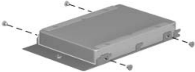
Figure C-11. PM3.0 × 3.0 Screw Locations
