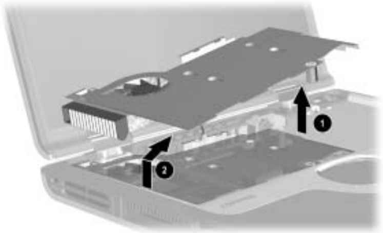
Figure 5-22. Removing the Heat Spreader
