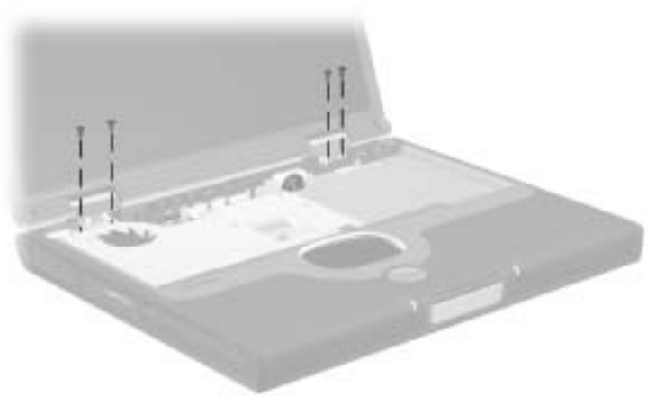
Figure C-14. TM2.5 × 9.0 Screw Locations
