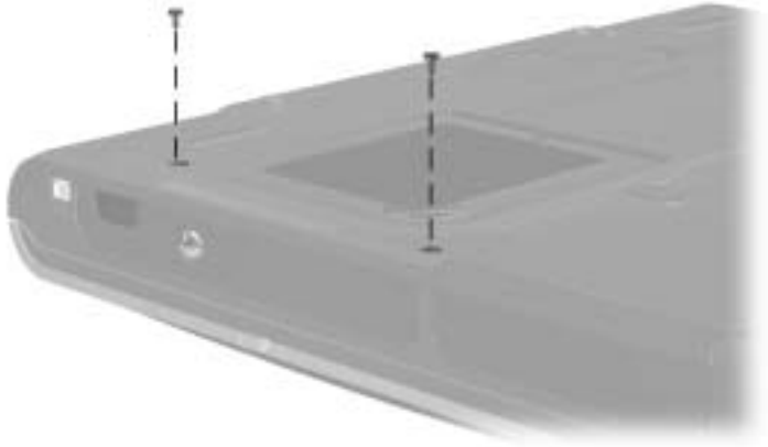
Figure C-1. TM2.5 × 5.0 Screw Locations
