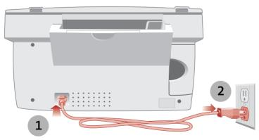
You should plug the power cord, which has a three-wire electrical grounding type plug, into a grounded electrical outlet.
