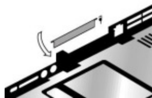
Figure 2-21. Removing a PCMCIA Door
