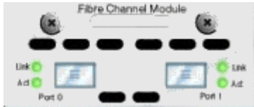
Figure 4-18: Fibre Channel module image
