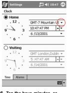
6 Tap the hour, minutes, or seconds to select the time you want to adjust 7 Tap the up or down arrow to adjust the time
