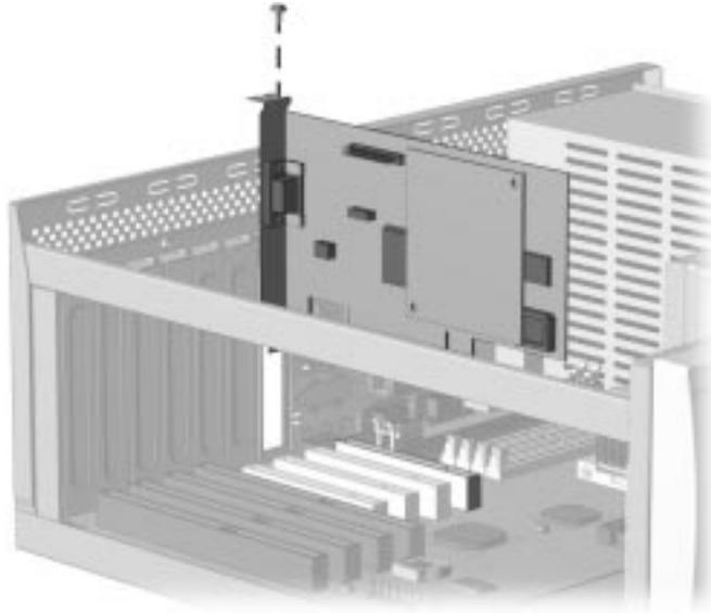
**Figure 5-5.** *Removing a Board*
