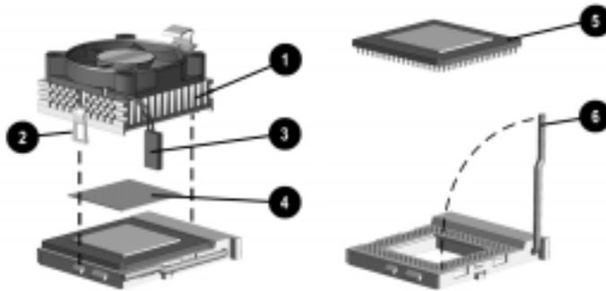
*Figure 5-13.2. Removing the Microprocessor from the System Board*
