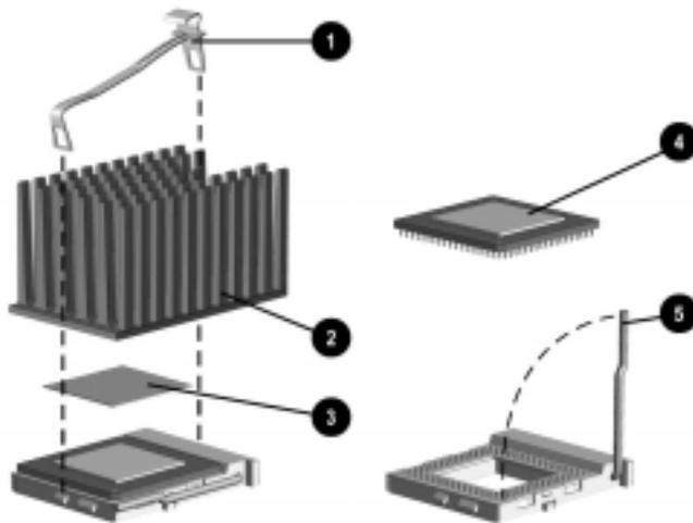
**Figure 5-13. Removing the Microprocessor from the System Board**
