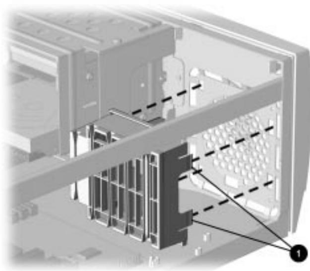
**Figure 5-6.** *Removing the Expansion Board Guide*
