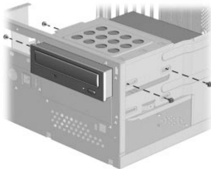
**Figure 5-23.** Removing a 5.25-Inch Drive
