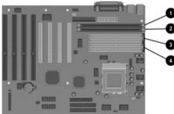
**Figure 5-9.** Memory Module Sockets on the System Board
