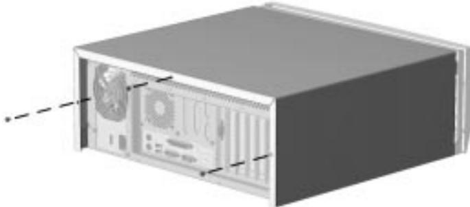
*Figure 5-3. Removing the System Unit Cover*
