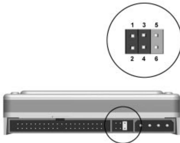
**Figure 6-3.** 1.6-GB EIDE Hard Drive Jumper Settings
