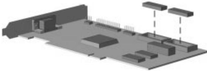
**Figure 5-8.** *Installing a Graphics Module*
