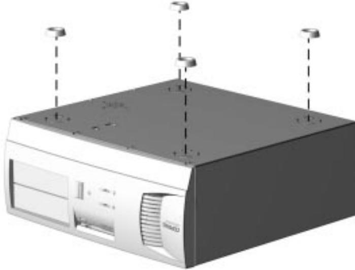
*Figure 5-2. Installing the Feet*
