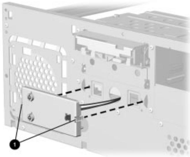
**Figure 5-15.** Removing the LED Retainer Assembly and Cables
