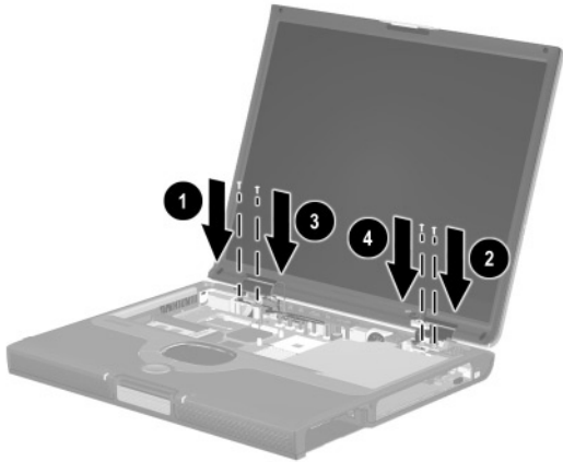
Figure 5-26. Installing the Display Screws
