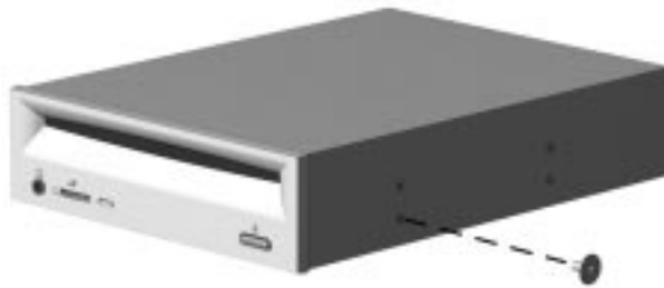
Inserting the High Hat Screw on the Right Side of the Drive
