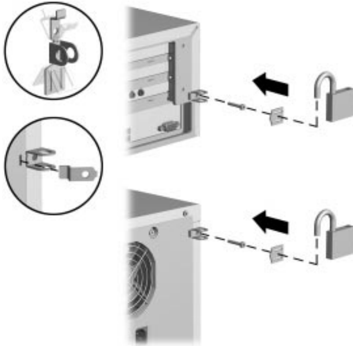
Installing the Cable Lock Provision and Padlock
