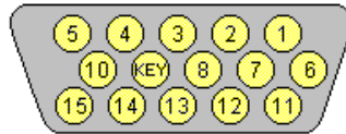
Figure 6-2. VGA Monitor Connector, (Female DB-15, as viewed from the rear of chassis).
