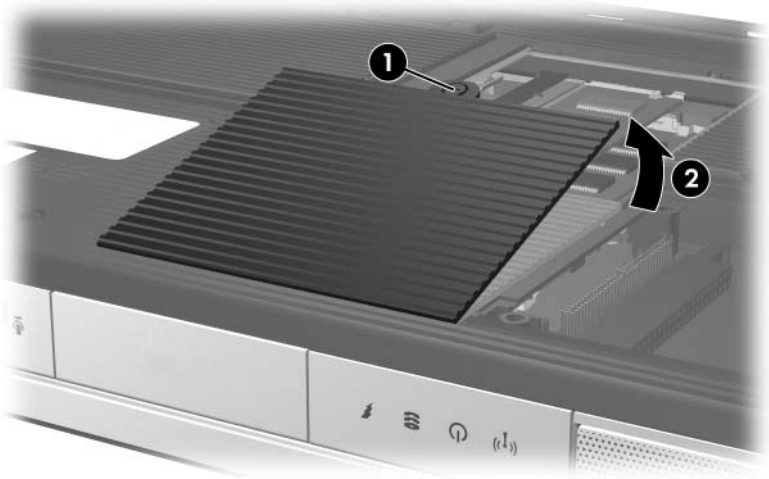
Removing the Mini Card Compartment Cover
