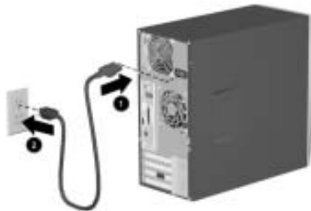
reconnecting the power cable on the S0000/8000 (S0000 shown)
