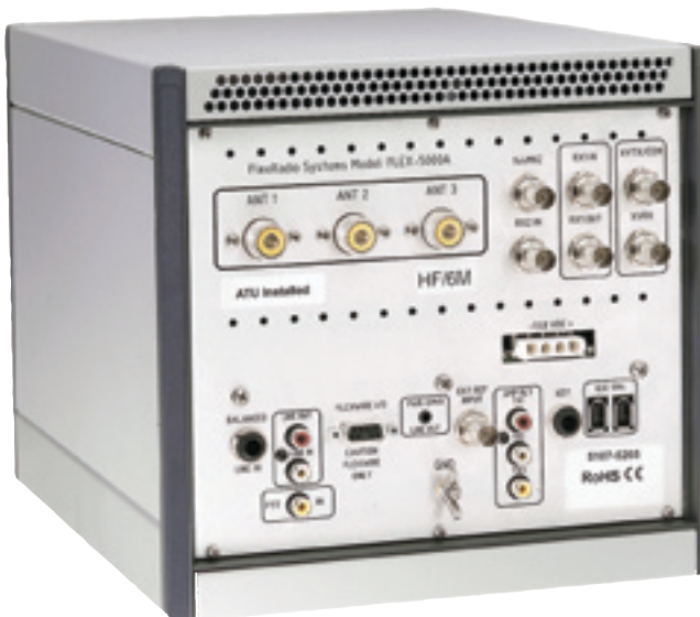
Figure 4 — Rear view of the Flex-5000A. Note the real analog connectors here.
