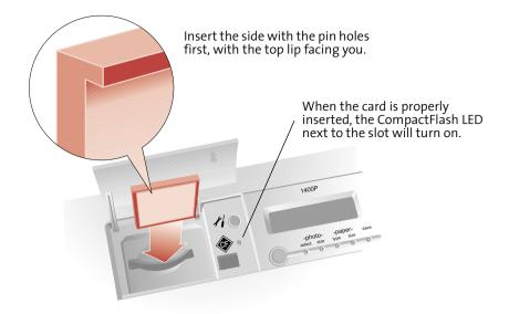
**WARNING**: Never remove the memory card when the CompactFlash light is flashing, or you could damage the card.
