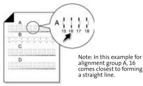
Using the same **Up**, **Down** and **Enter** buttons used in step 4, change the value for the letter displayed on the printer LCD, and then press Enter to select it. The next alignment letter will be shown until you have set all the alignment values for the page.
