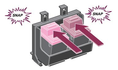
1 Push **back** on the cartridges until they *snap* securely into place.
