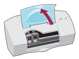
When you raise the front cover, the print cartridge carrier moves to the loading position.
