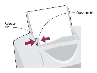
Squeeze the release tab and paper guide together and slide the paper guide to the edge of the paper.
