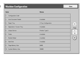
On the [Machine Configuration] screen, you can check the following items.
