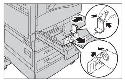
**3** Load the paper with the side to copy or print on facing up. Align the leading edge of the paper with the left side of the tray.
