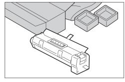
**6** Peel the protective sheet off the new drum cartridge.
