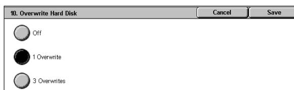
When copy (P.49), fax (P.99), scan (P.165), or print (P.234) processing is completed, the data is deleted from the hard disk and the area on which the deleted data was stored is automatically overwritten with blank data. This feature prevents unauthorized retrieval or restoration of the data recorded on the hard disk. It also applies to copy source, and other information stored temporarily by the system.
