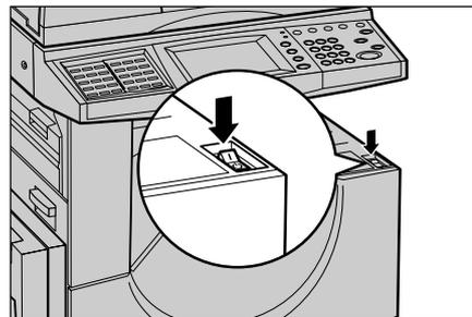
**Note** • When the power does not come on, check if the power cord is plugged into the power outlet and the <RESET> button is in a reset state (button is pressed in).
