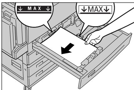
When loading paper in the Tandem Tray Module, align the paper against the left back corner of the tray.
