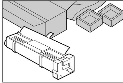
**7** Place the drum cartridge on a flat surface. Undo the sealing tape as shown, and carefully pull it out to remove the protective sheet out of the cartridge.
