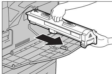
**4** Remove the new toner cartridge out of the box and shake it from side to side before removing it out of the bag.
