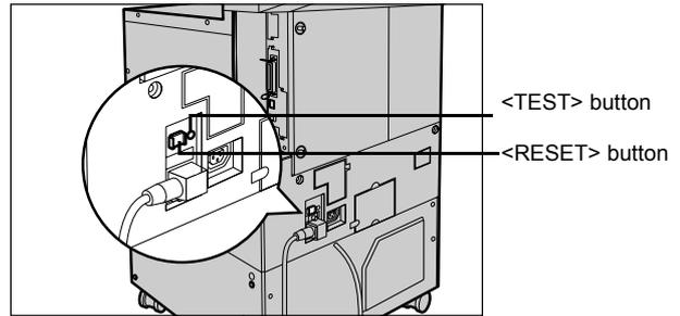
Once a month, check the breaker for correct operation. Also, make sure that it is earthed. If not, the breaker cannot detect current leakage which can cause electric shock.
