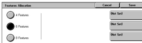
**Note** • The position of the buttons on the right of the screen shows the position of the buttons in the [Copy] screen.
