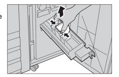
4 Hold the left and right tabs on the new staple cartridge to return the cartridge to its original position, and gently push the cartridge until it clicks into place.
