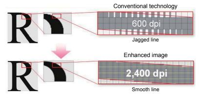
This printer reproduces smooth lines and gradations by  $1200 \times 2400$  dpi high-resolution LED print heads and Micro Accurate Control Screen (MACS) Technology.
