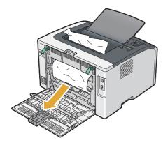
4 If no paper is found in the paper path, remove any paper jammed from the center output tray.
