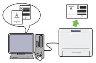
The multiple up print feature allows you to print multiple pages on a single sheet of paper. This feature helps reduce paper consumption.
