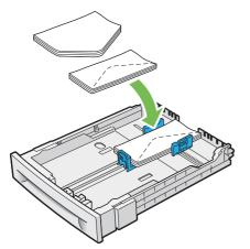
To prevent DL and Monarch from being wrinkled, they are recommended to be loaded with the flaps opened. Place the print side facing up, and the flaps come at the bottom when you face towards the printer.
