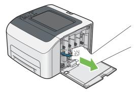
7 Insert the print head cleaning rod fully into the hole beside the arrow on the printer until its tip reaches the interior of the printer as illustrated below, and then pull it out.
