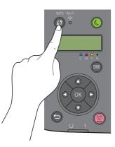
2 Start the WPS operation on the wireless LAN access point (Registrar) or router within two minutes. When WPS is successful, the r (Wi-Fi) LED lights up. The wireless connection is established and setup for wireless LAN is complete.
