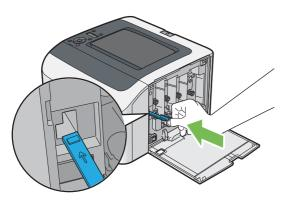
**10** Replace the black toner cartridge by adjusting it to the associated cartridge holder, and then insert it firmly by pressing near the center of the label until the toner cartridge clicks.
