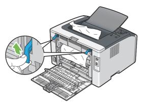
3 Remove any paper jammed from the rear of the printer by carefully pulling it in the direction of the arrow shown in the following illustration.
