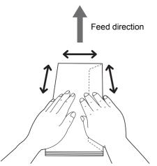
If envelopes are still not fed correctly, curl the edge of the envelopes as shown in the following illustration. The amount of the curl should be 5 mm (0.20 inches) or less, 2 or 3 mm (0.08 or 0.12 inches) is recommended. The area of the curl should be 8 – 10 mm (0.32 – 0.39 inches) from the top edge of the envelopes. Do not curl the envelopes too much or make a crease.
