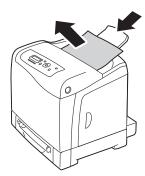
3 Pull the standard 250-sheet tray out of the printer about 200 mm. Hold the standard 250-sheet tray with both hands, and remove it from the printer.
