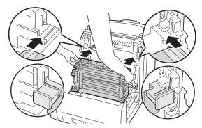
9 Turn the four drum cartridge lock levers 90-degrees clockwise to lock the drum cartridge.
