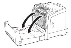
4 Turn the four drum cartridge lock levers 90-degrees counterclockwise.
