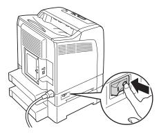
2 Disconnect the power cord from the power connector on the rear of the printer.
