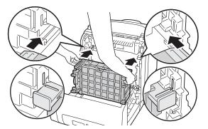
6 Turn the four drum cartridge lock levers 90-degrees clockwise to lock the drum cartridge.
