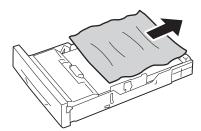
3 Pull the jammed paper out carefully to avoid tearing it. If you cannot remove the paper, go to the next step to remove the jammed paper from the inside of the printer.
