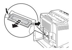
4 Hold the memory module and pull it straight out.
