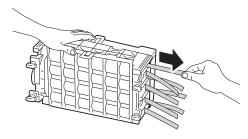
4 Remove the rear protective cover from the drum cartridge.
