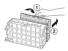
5 Insert the drum cartridge until the line on the handle aligns with the white line on the printer.
