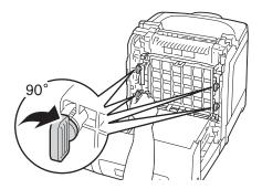
7 Remove the front protective cover from the drum cartridge.
