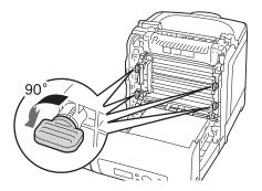
6 Hold the drum cartridge levers, and then pull out the drum cartridge.
