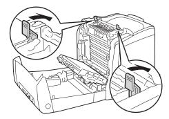
7 Confirm that there are no scraps of paper remaining inside the printer, and then close the belt unit.
