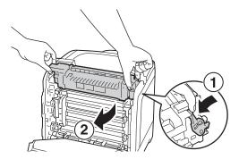
6 Hold both sides of the fuser unit. Next, slightly raise the right side while holding down the left side, and slide out the fuser unit.
