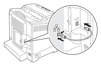
To connect the printer to the network, connect one end of the Ethernet cable into the Ethernet port on the rear of the printer, and the other end to a LAN drop or hub.
