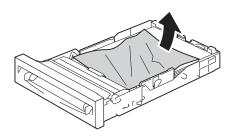
Pull the jammed paper out carefully to avoid tearing it. If you cannot remove the paper, go to the next step to remove the jammed paper from the inside of the printer.
