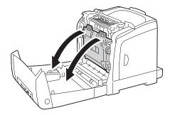
4 Lift the levers at both ends of the fuser unit, and remove the jammed paper. If you are still unable to remove the paper, go to the next step.
