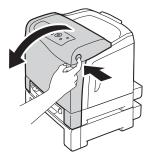
Open the belt unit until it stops and remove the jammed paper. Confirm that there are no scraps of paper remaining inside the printer.
