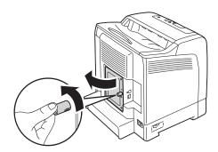
3 Push the clips on both sides of the slot outward.
