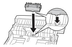
Insert the feed roller unit into the axle until it snaps. The protrusions fit completely into the slots and the roller hook reseats into the groove on the axle.
