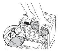
2 Push the fuser unit forward until the right groove of the snaps into place.
