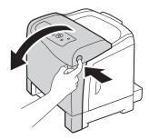
Open the belt unit until it stops and remove the jammed paper. Confirm that there are no scraps of paper remaining inside the printer.
