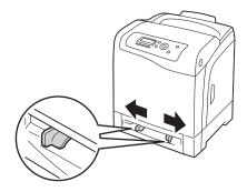
2 Hold both sides of the print media face down close to the SSF, and push it 8 cm to 9 cm (4 inches) into the printer until it automatically feeds.
