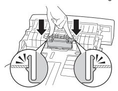
3 Load paper in the standard 250-sheet tray, and then insert the standard 250-sheet tray into the printer and push until it stops.
