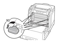
5 Hold the drum cartridge levers, and then pull out the drum cartridge.
