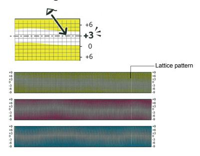
Using the operator panel, enter the values found in the color registration chart to make adjustments.
