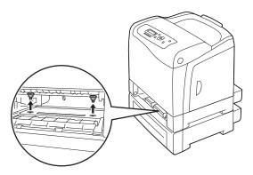
Gently lift the printer off the optional 250-sheet feeder, and place it on a level surface.
