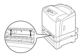
8 Insert the standard 250-sheet tray into the printer, and push until it stops.
