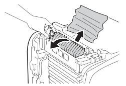
6 Close the cover of the fuser unit and press down the levers at both ends of the fuser unit.
