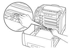
8 Insert the drum cartridge until the line on the handle aligns with the white line on the printer.
