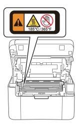
Push down the lock lever and take the toner cartridge out of the drum unit. Remove the jammed paper if there is any inside the drum unit.
