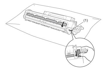
Wipe the surface of the drum gently with a dry cotton swab until the dust or glue on the surface comes off.
