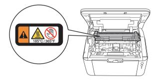
5 Push down the lock lever and take the toner cartridge out of the drum unit. Remove the jammed paper if there is any inside the drum unit.
