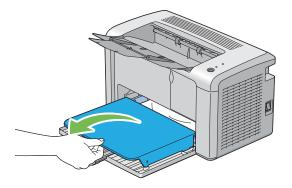
2 Remove any paper jammed from the front of the printer.
