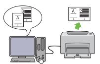
Duplex Print is to print two or more pages on the front and back sides of a single sheet of paper manually. This feature allows you to reduce the paper consumption.
