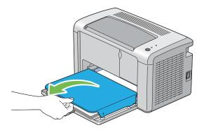
**5** Remove any paper in the multipurpose feeder (MPF). Keep the paper wrapped and away from humidity and dirt.
