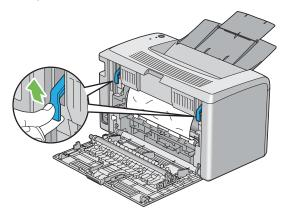
3 Remove any paper jammed from the back of the printer.
