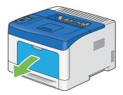
6 Grasp both sides of the bypass tray, and then pull the bypass tray from the printer.
