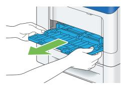
Pull the standard 250 sheet tray out of the printer about 200 mm. Hold the standard 250 sheet tray with both hands, and remove it from the printer.
