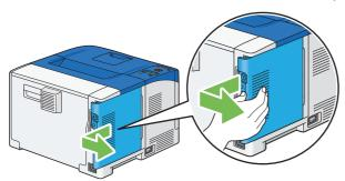
4 Hold the edge of the memory module with the labeled side down and the connector toward the control board, and then insert it into the slot.
