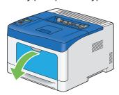
2 Grasp both sides of the bypass tray, and then pull the bypass tray from the printer.
