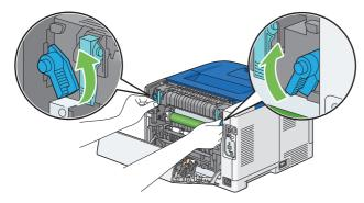
4 Grasp the grips on both sides of the fusing unit placing thumb on the knurling, and then pull out the unit.
