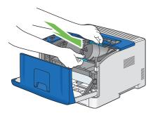
3 Make sure that the two tabs of the toner cartridge align with the grooves on the printer, and then insert it into the printer until it clicks.
