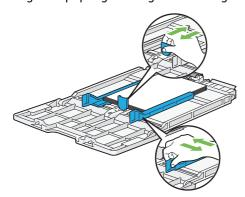
7 Insert the bypass tray into the printer.
