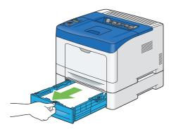
2 Hold the optional 550 sheet feeder with both hands, and remove it from the printer.
