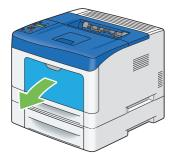
4 Grasp both sides of the bypass tray, and then pull the bypass tray from the printer.
