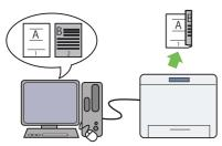
The 2-Sided Print feature is to print two or more pages on the front and back side of a single sheet of paper. This feature helps reduce the paper consumption.
