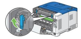
3 Slide the envelope switches on both sides of the fusing unit to the 🔋 position.
