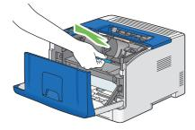
5 Grasp the handle on the top of the drum cartridge with the other hand, and then pull it out completely.
