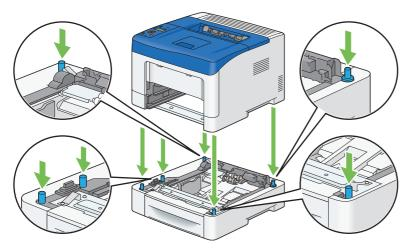
10 Secure the optional 550 sheet feeder to the printer by tightening the two screws provided with the feeder with a coin or similar object.
