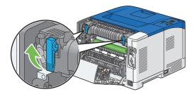
3 Slide the envelope switches on the both sides of the fusing unit to the 🛢 position.
