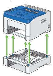
8 Insert the standard 250 sheet tray into the printer, and push until it stops.
