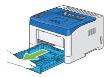
8 Hold the standard 250 sheet tray with both hands, and remove it from the printer.
