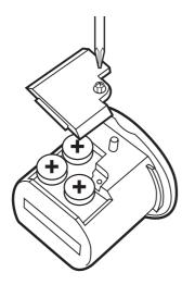
Insert three (3) LR44 "button cell" batteries. Be sure that the "+" sign is facing you. Replace the battery compartment door and tighten the screw.
