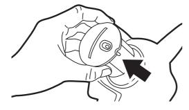
Using a Phillips® screwdriver, loosen the screw in the battery compartment door located on the side of the voice unit and remove the battery compartment door.
