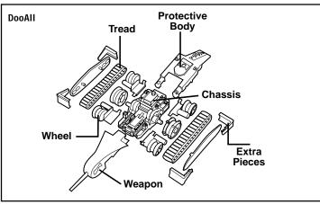
Start with the basic chassis and add the drive system by snapping the pieces together as shown.
