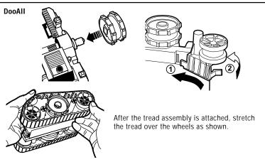
After the drive system is assembled, you can attach the Bot's offenses. Simply slide the attachment into place on the chassis as shown, and insert fully.
