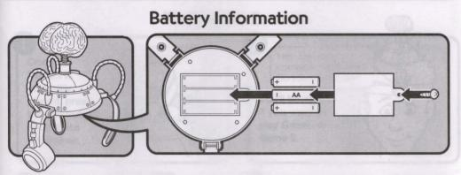
Loosen the screw on the battery compartment (located on the underside of the helmet), and remove the door. Insert 3 "AA" size batteries (we recommend alkaline), making sure to match the + and - symbols with the markings in the plastic. Then replace the door and tighten the screw.
