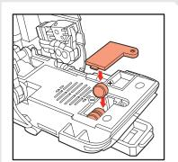
Using a Phillips/crosshead screwdriver (not included), loosen screw in battery compartment door. Remove door. Insert 3 fresh A-76 button cell batteries. Replace door, and tighten screw.
