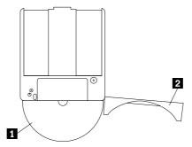
To return the disc to the cartridge, align the label side of disc **1** with the DVD-RAM cartridge label side. Insert the disc and close the cartridge lid **2**. A clicking sound will ensure the lid door is closed.
