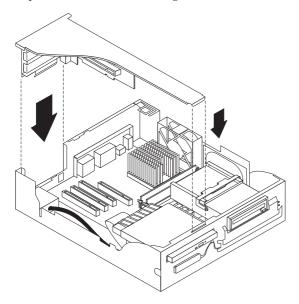
8. Replace the cover and connect the cables. Refer to your system user's guide for details on replacing cover and connector cables.
