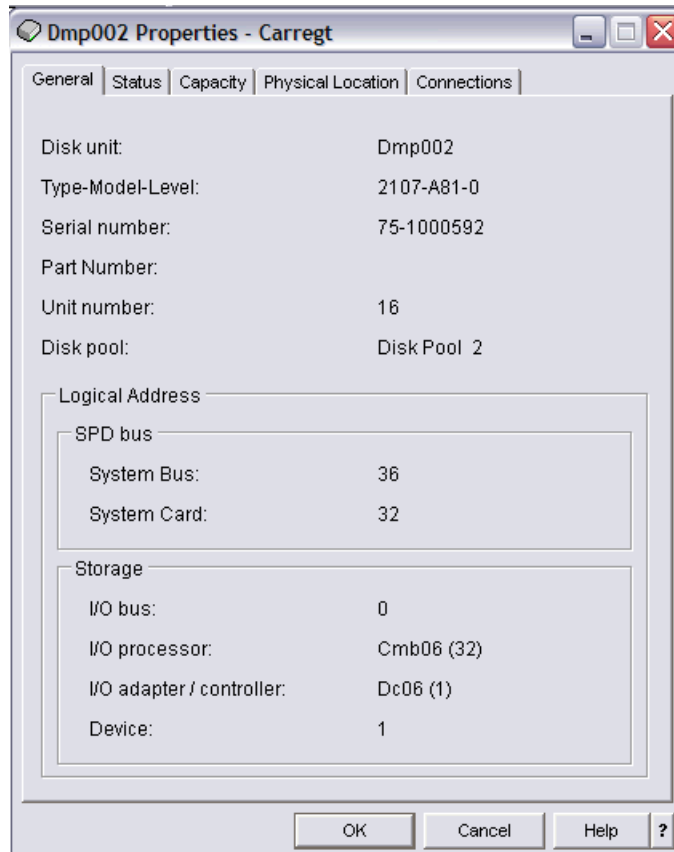
Figure B-32 Multipath logical unit properties
