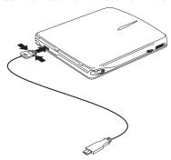
Make sure that the metal plate on the smaller connector is facing up when you plug it into the USB connector on the CD-ROM drive.
