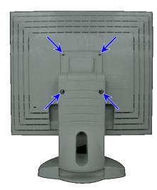
Remove the four mounting plate retaining screws. One screw at each corner. Lift the base up and away from the monitor.
