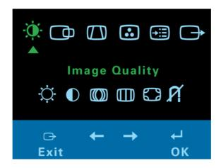
Each sub-menu icon is selected by highlighting it via the "←" "→" control and pressing button "←" to select. To exit the main or sub-menu then press the exit button "←".
